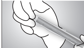
3 - If probe cover gathers too tightly, pull "Grip Tip" off of colonoscope to free up
